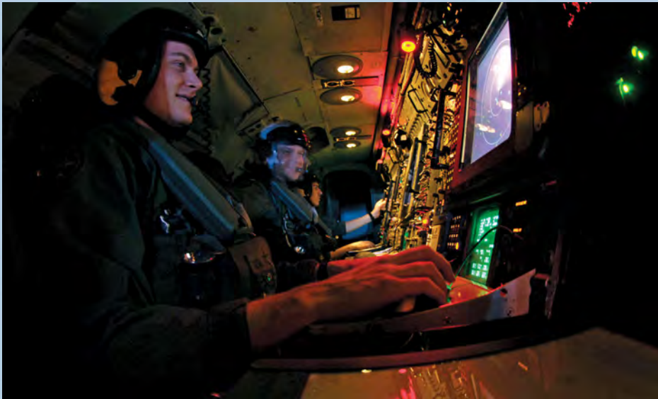
Above: The Hawkeye's Combat Information Center provides three identical mission system operator positions for the Radar Operator (RO), Combat Information Center Officer (CICO) and the Air Control Officer (ACO) US Navy/MCS Kyle D. Gahlau
