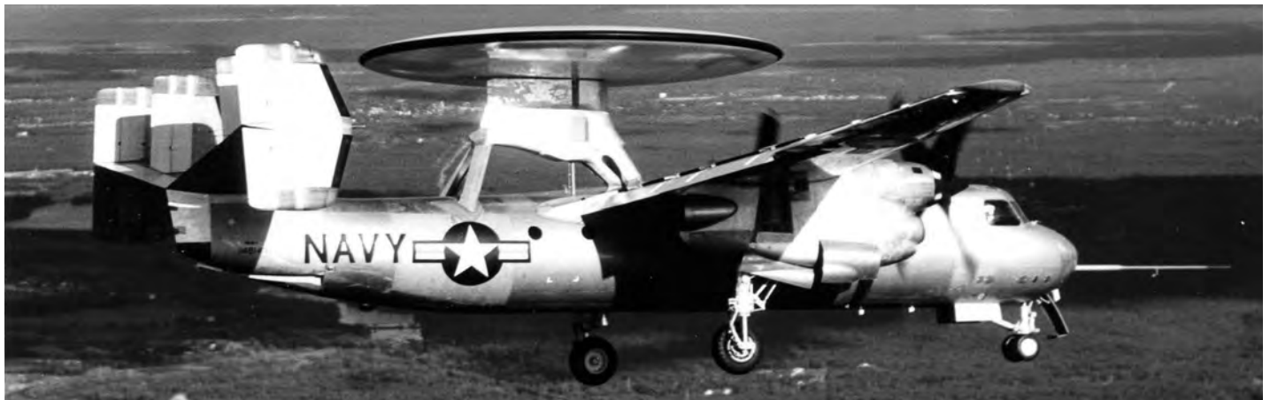
The prototype Hawkeye first flew on October 21, 1961, under the designation W2F-1. Assigned Bureau Number 148147, it was later modified to become the prototype C-2A carrier on-board delivery (COD) prototype Northrop Grumman
