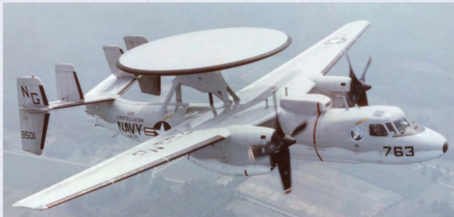
The Baseline E-2Cs featured the AN/APS-120 and then the AN/APS-125 radar and AN/ALR-59 Passive Detection System (PDS). The E-2C entered service with VAW-123 in November 1973 and Grumman produced 69 over a ten-year period Northrop Grumman
