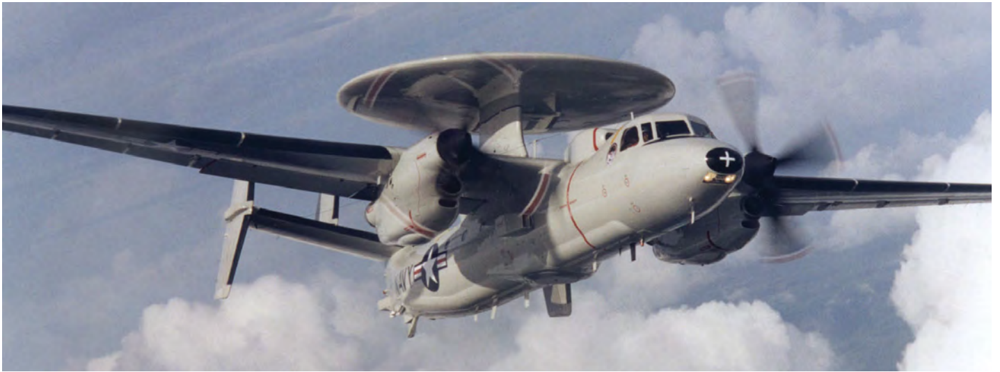
First flown in June 1998 the E-2C Hawkeye 2000 featured numerous upgrades that included the AN/USG-3 Cooperative Engagement Capability (CEC). Northrop Grumman delivered the first of this variant in 2002 and eight-blade Hamilton Sundstrand NP2000 propellers were introduced in production in mid-2004 Northrop Grumman
