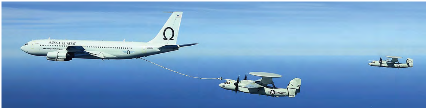
An E-2D operated by air test and evaluation squadron VX-1 conducts refuelling with a KC-707 operated by Omega Aerial Refueling Services near NAS Patuxent River, Maryland. The first E-2D equipped for this was delivered to VAW-120 in September 2019 US Navy
