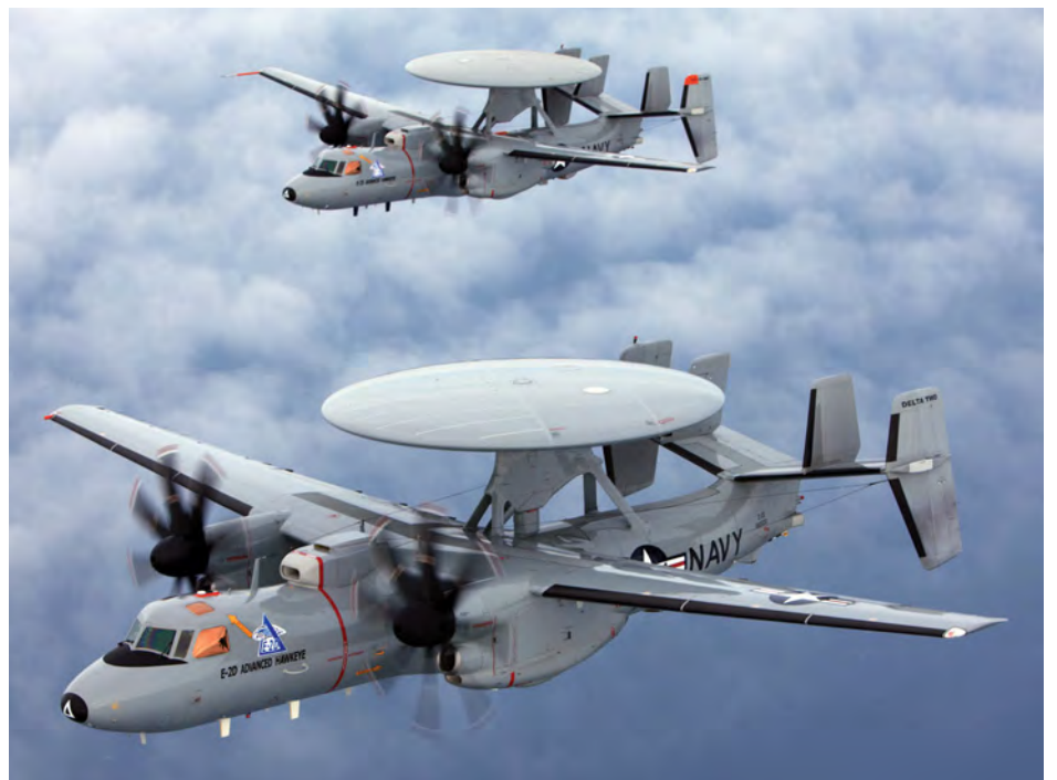
First flown on August 3, 2007, the E-2D Advanced Hawkeye features the AN/APY-9 advanced electronically scanned array radar, enhanced AN/ALQ-217A electronic support measures (ESM) system and upgraded AN/USG-3B Cooperative Engagement Capability (CEC) Northrop Grumman
